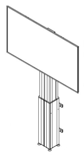
Motorized Wall/Floor support for large size and touch screens up to 100" and 150Kg.
