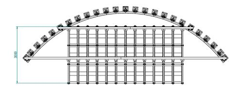
This solution is designed to guarantee perfect alignment of the LED tiles, thanks to the adjustments of the X, Y and Z axes.
