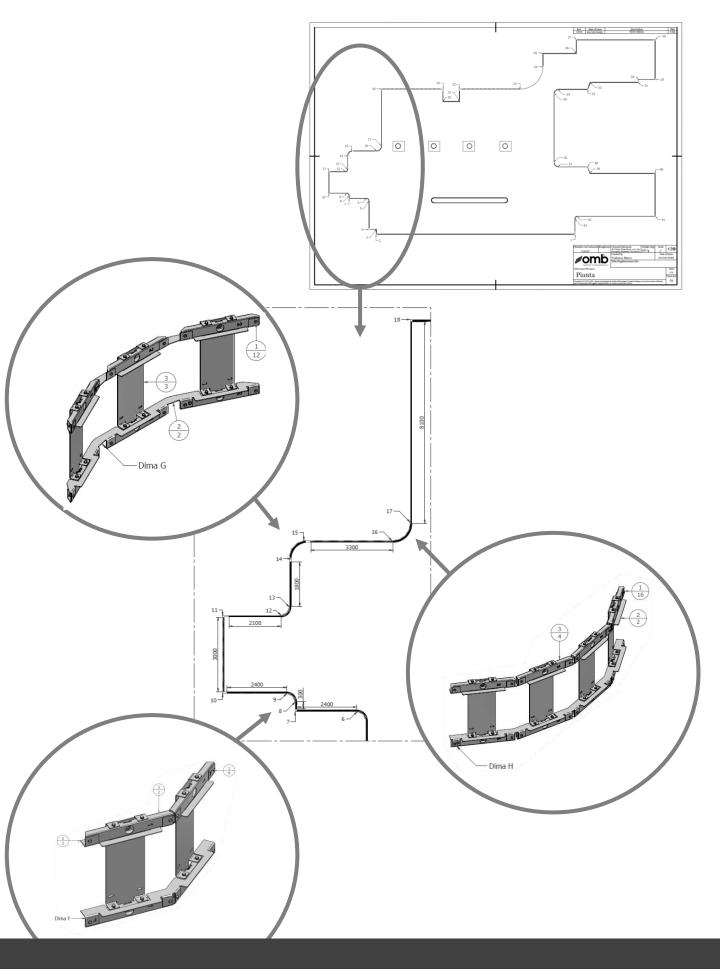
When the complexity of the structure is too high, OMB can offer the pre-assembled structure
