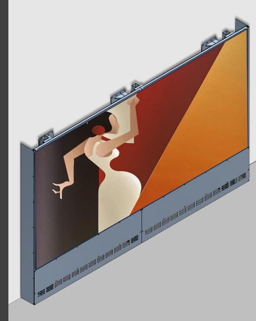
The dvLED structures are customized based on the total size of the LED and the model/brand of tile used
